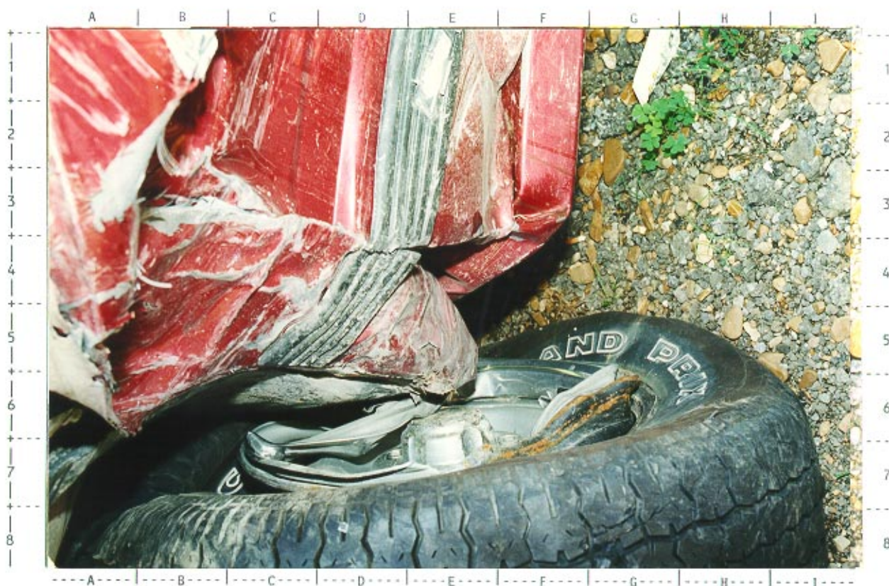
# 69 -- Close-up of direct damage to 1988 Chevrolet pickup's LF rim and also behind displaced left front wheel--viewed from left
